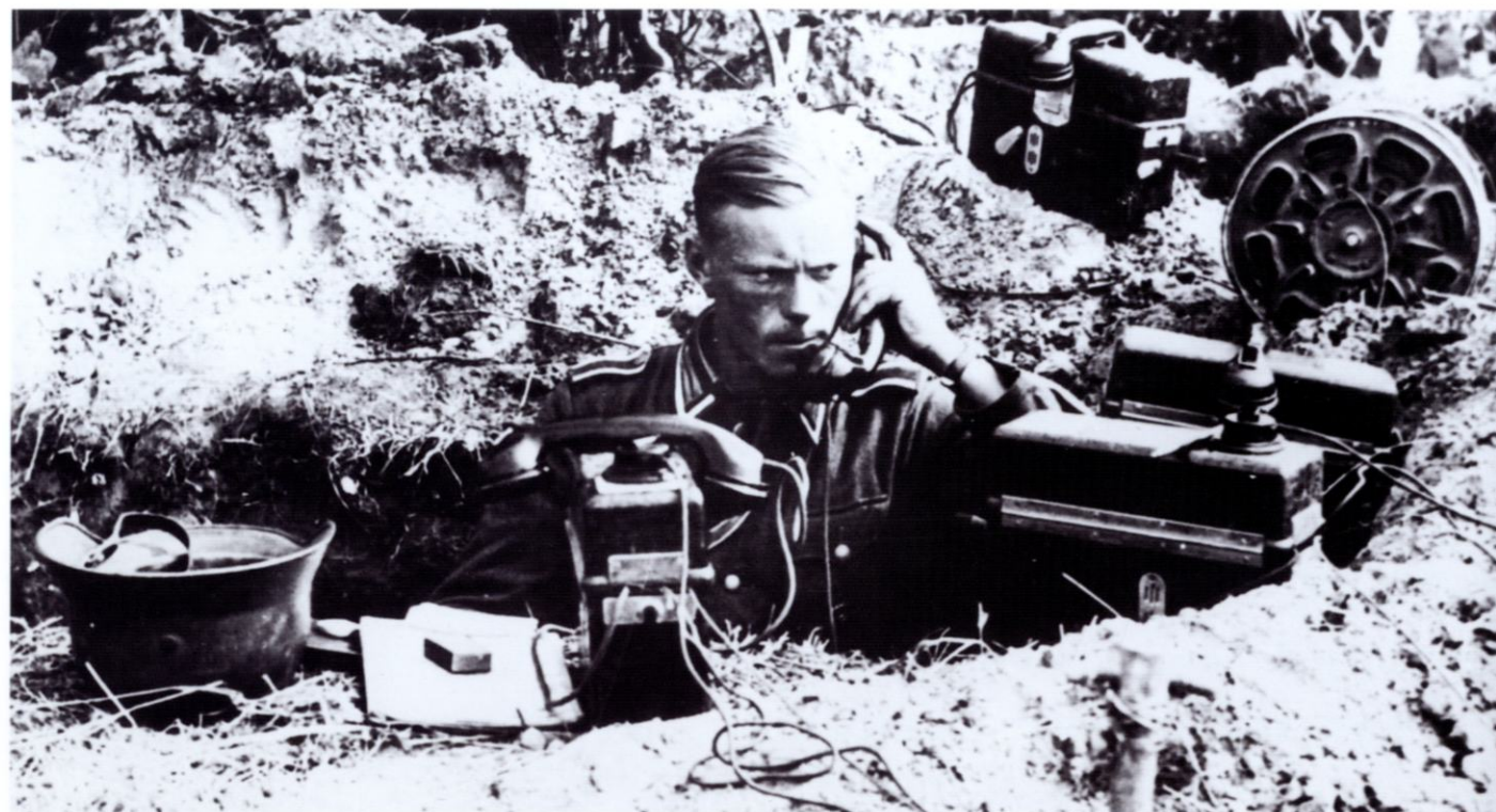
Above: Field telephones with landlines were widely used as they were far more secure than wireless; however, as the narrative tells, they were liable to damage from shell fire. (Brian L. Davis Collection)
